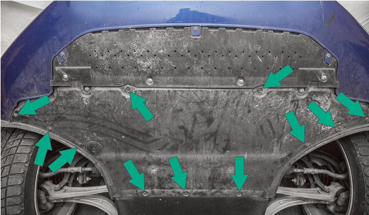
Remove belly pan from vehicle by sliding backwards.
