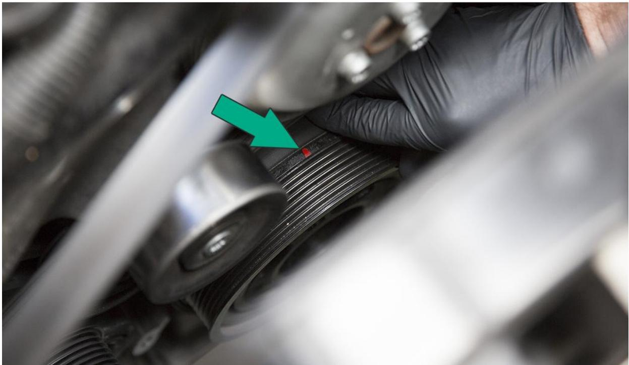
Using a 6mm hex bit, break loose and remove all 8 bolts securing the crank pulley to the crankshaft. Remove pulley.
