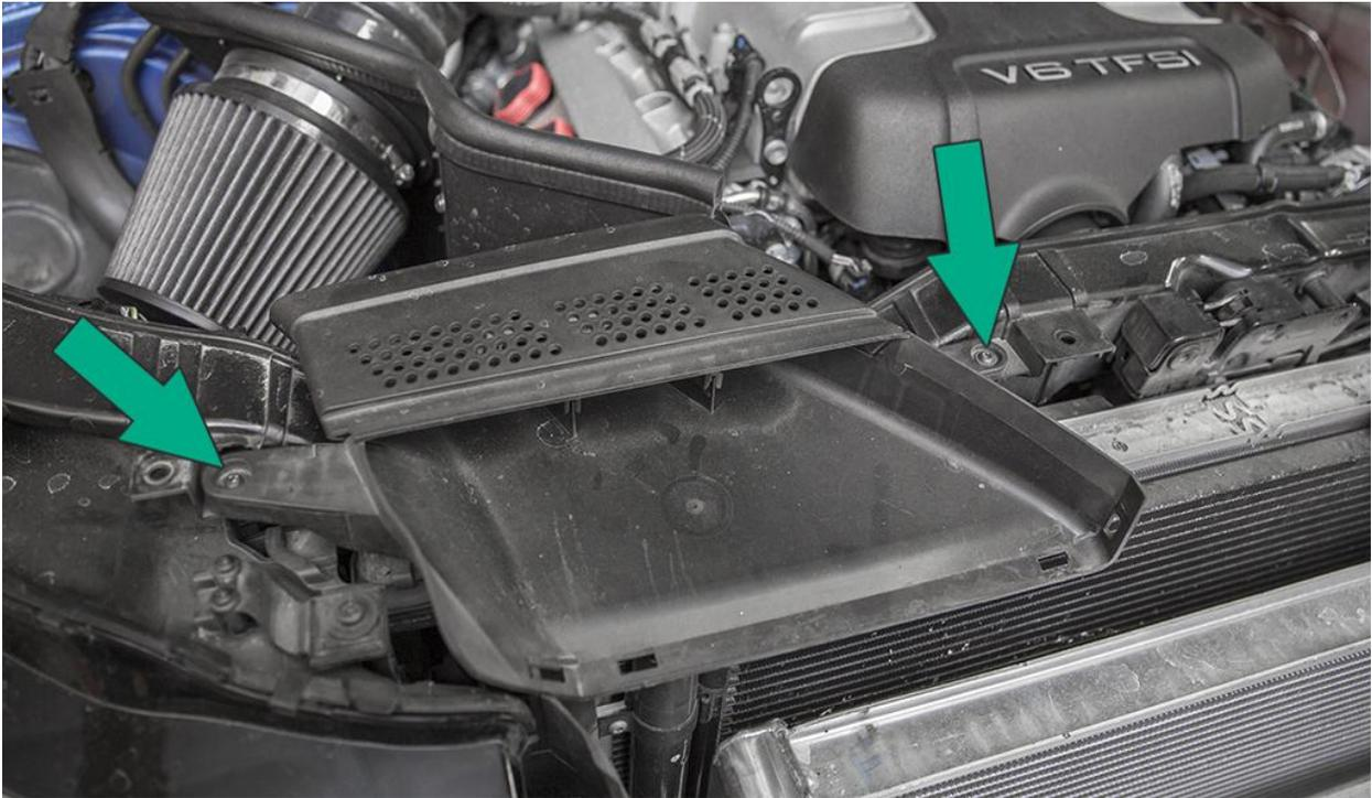
Remove the two T30 radiator support to fender bolts, one is located on each side above the headlights.
