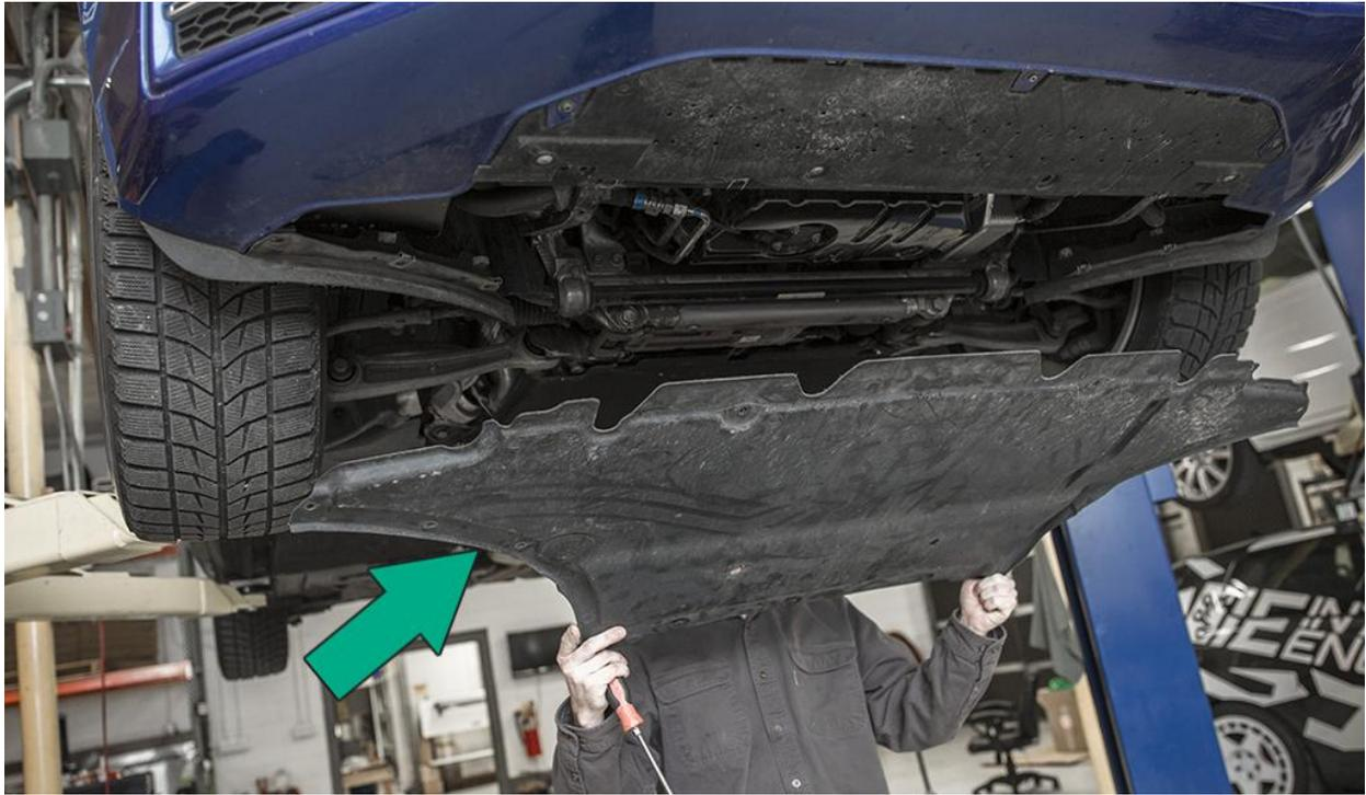
Remove the six T30 torx screws from the underside of the bumper that secures it to the radiator support.
