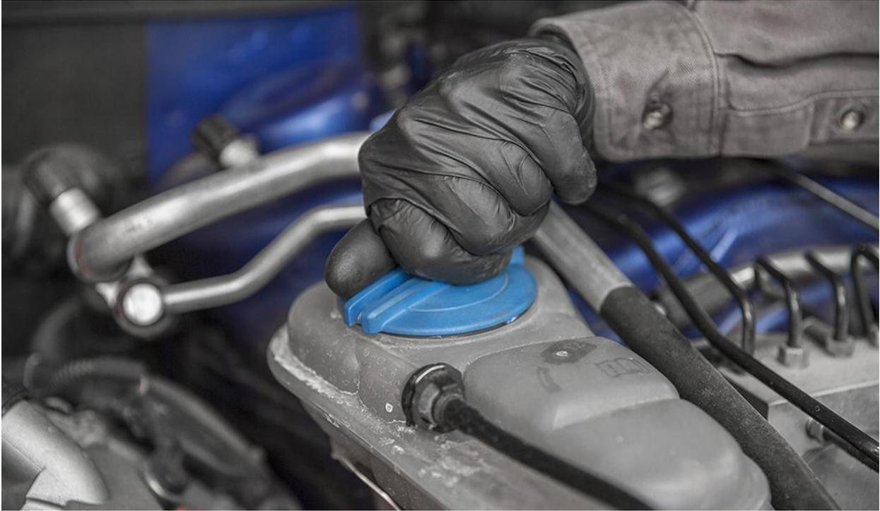
Using a small flathead, release the coolant overflow line spring clip. Gently pull back on the line to release it from the coolant tank.
