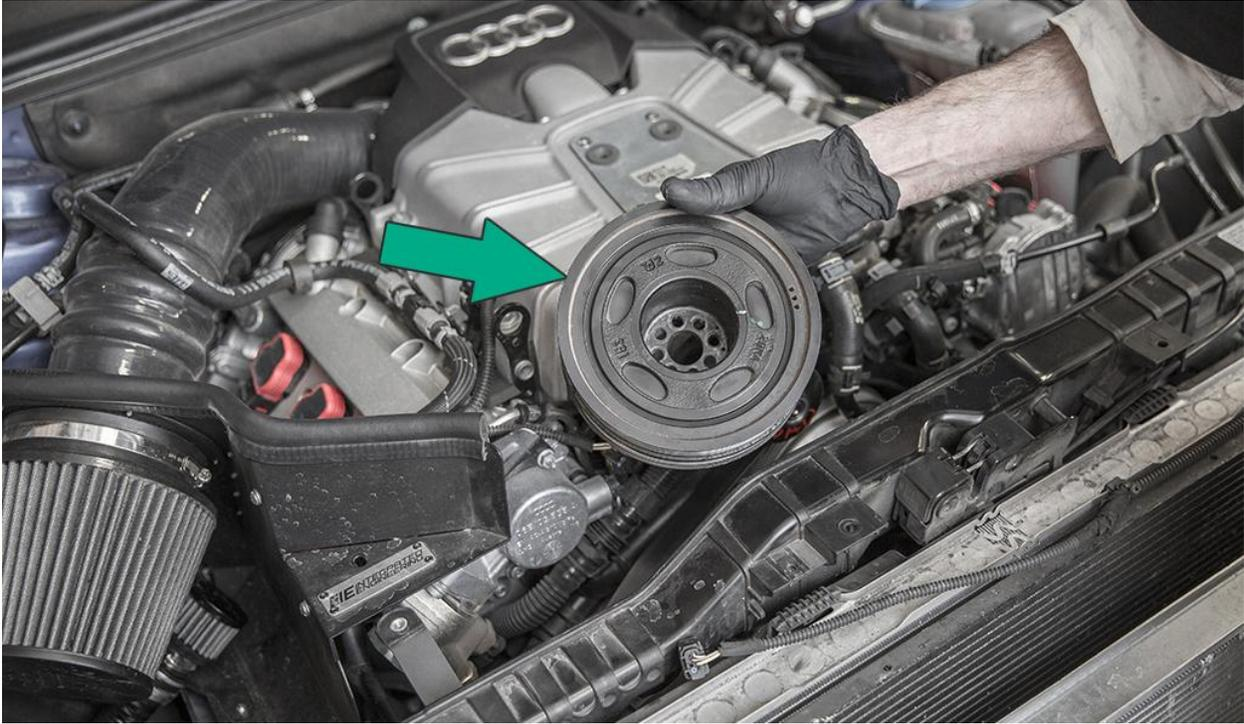
To the side of the pulley there is a mount post on the engine block. Using an angle grinder and grind wheel, remove roughly 3-4mm of material from this post to make room for the larger pulley and belt. This post is not used to mount anything on this engine.
