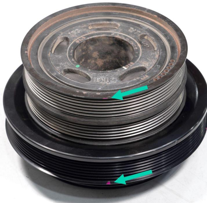
Install the pulley into the car, making sure the paint pen mark up is lined up vertically, same as uninstal, then apply blue loctite to the new supplied bolts and slide them into place through the pulley.
