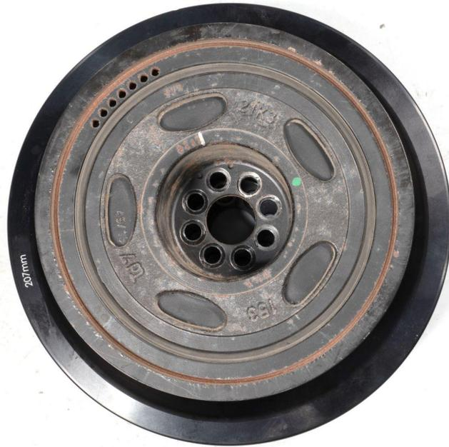
Once the offset holes are aligned, mark the IE pulley with a paint pen in the same location as your paint mark on the factory pulley, so you know which side of the pulley needs to be facing directly up.
