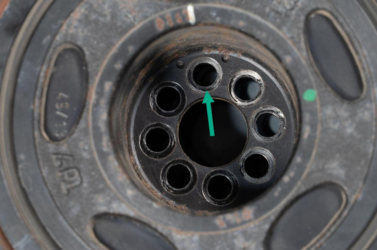
Using the identifying marks in the previous step, line up the offset holes and place the factory pulley on top of the IE pulley making sure all bolt holes line up.
