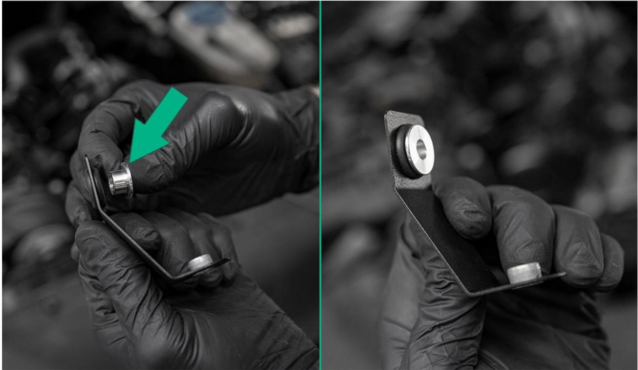
Using a T30 Torx driver and included screw, install the front support bracket to the radiator support as seen below.
