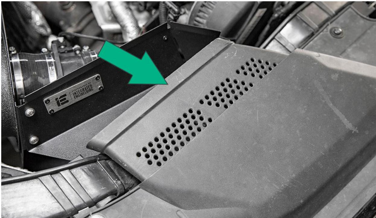
Install the trim seal at one end of the heat shield and push down firmly on the seal to lock it into place around the edge.
