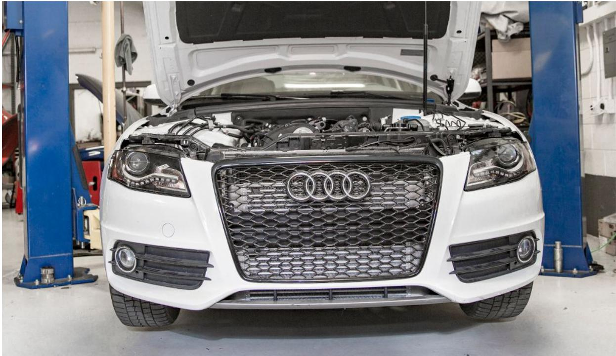
Start the installation procedure by removing the stock engine cover, pull up on the corners to release the grommets and set aside.
