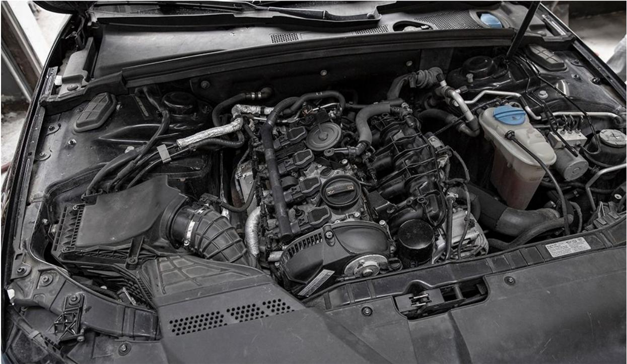
Carefully disconnect the MAF harness from the MAF housing by pushing down on the clip and pulling back.
