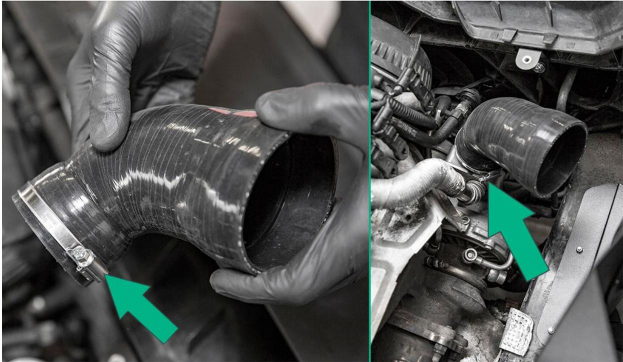
Install 80-100mm clamp onto the large side of the heatshield silicone and place onto the velocity stack. Tighten clamp with screwdriver.
