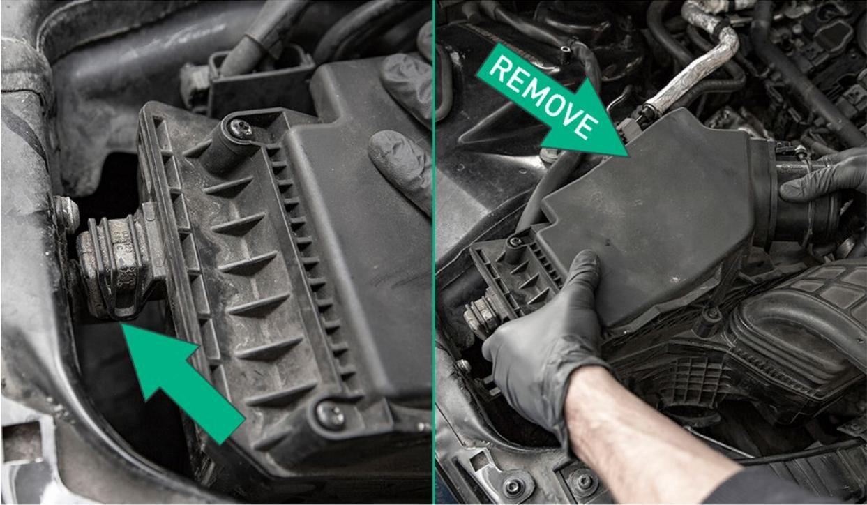
Pull to remove both factory rubber grommets from the bottom side of the airbox. Set these aside as you will reuse them later.
