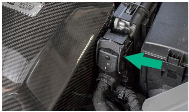
Check space between the ECU harness and air box, the fitment is tight. If they look to be making contact, loosen the mount tab bolt and pull the intake to free up some room.
