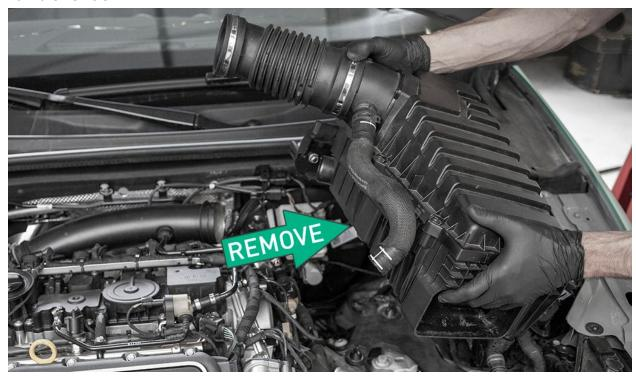
Using a sharp pair of dikes, cut the hose clamp from the intake to evap breather hose and remove it from the one-way valve.
