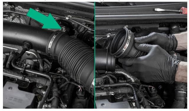
Pull up around the edges of the air box to release it from the push grommets, then remove it from the vehicle.
