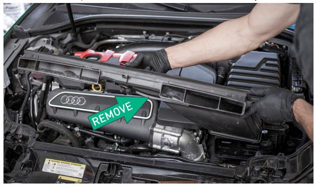
Carefully remove the engine cover by pulling up on the sides firmly to release it from the push-grommets.
