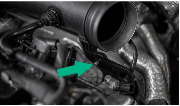
Using a hose clamp tool or pliers, release tension from the turbo to turbo inlet clamp and remove turbo inlet pipe & silicone from vehicle.
