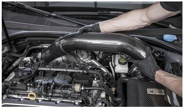
Loosely install the 3 remaining hose clamps to silicone couplers. Insert the intake pipe into the installed air box silicone coupler and push the opposite side silicone onto the turbo. **Do not tighten clamps in this step**.
