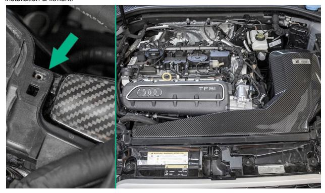
Loosely place the included 90-110mm hose clamp onto the airbox end of airbox silicone and install onto the rear of the integrated velocity stack. *Do not tighten clamp in this step.*
