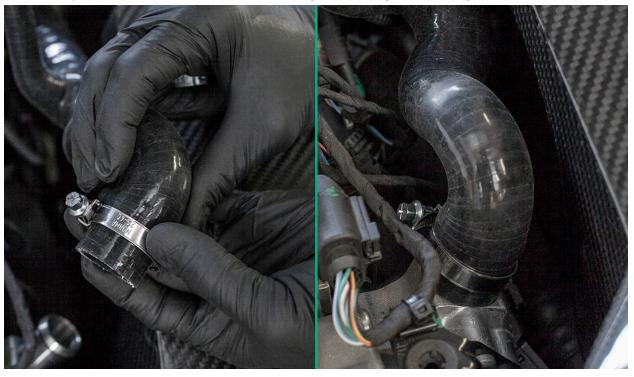
Install the OE-style clamp onto the evap breather silicone leg and install onto one way valve barb. *Do not tighten clamp in this step.*
