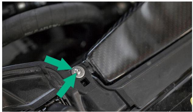
Reinstall ECU harness and push to seat the disconnect lever.
