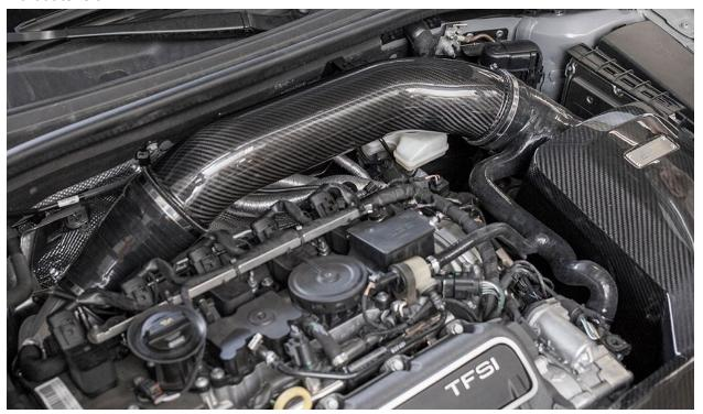
Once you are happy with the intake position, firmly tighten all 4 silicone hose clamps. *Do not over tighten hose clamps, doing so can damage your carbon fiber inlet.*
