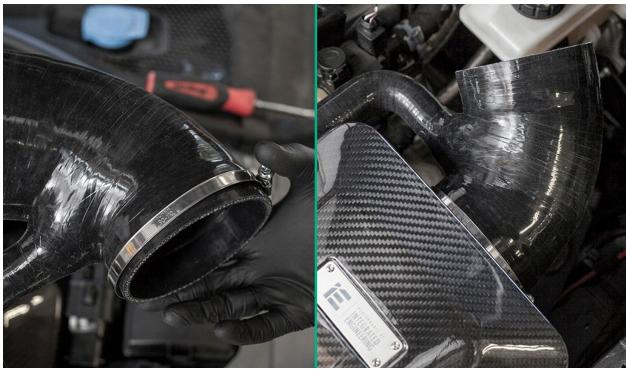
Install the small hose clamp onto the diverter silicone leg and install onto the diverter housing or (2019+ only) onto IE diverter adapter. *Do not tighten clamp in this step.*
