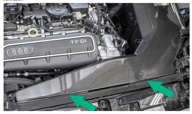
Line up the bottom intake plate push grommets with the factory mount posts, push down on the intake carefully to seat into place.
