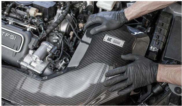
Verify the intake snorkel mount is under the factory cowel at the end to verify proper air box installation & fitment.
