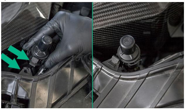
Line up the factory engine cover with the mount tabs, then push firmly to seat push grommets.
