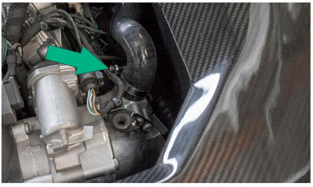
Using a pair of dikes, tighten the OE style hose clamp on the evap silicone line.
