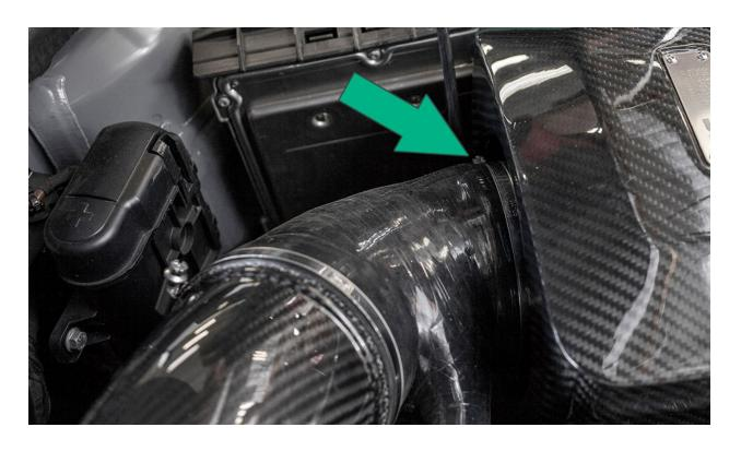
Tighten diverter valve silicone hose clamp.
