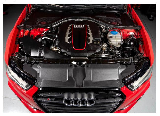
Remove engine cover by pulling straight up off the 4 alignment pegs
