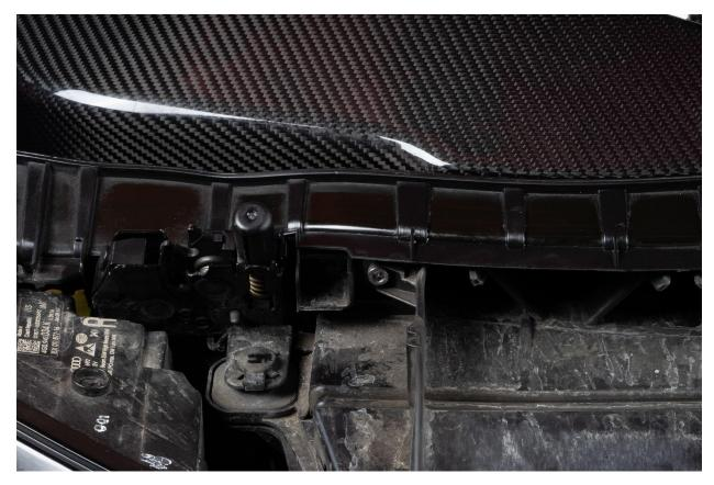
Reinstall radiator cover and secure in place with the push retainers, then reinstall engine cover.
