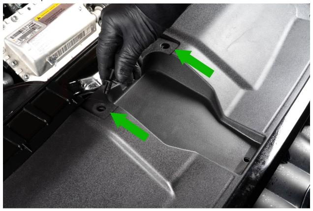
Pull up on front corners then out to remove radiator cover
